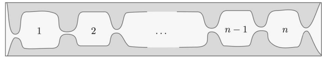
FIG. 1. Schematic of an array of n chaotic cavities. The cavities are connected via ballistic contacts with dimensionless conductance g_c . The semiclassical theory requires the limit g_c \rightarrow \infty at a fixed ratio n/g_c .
